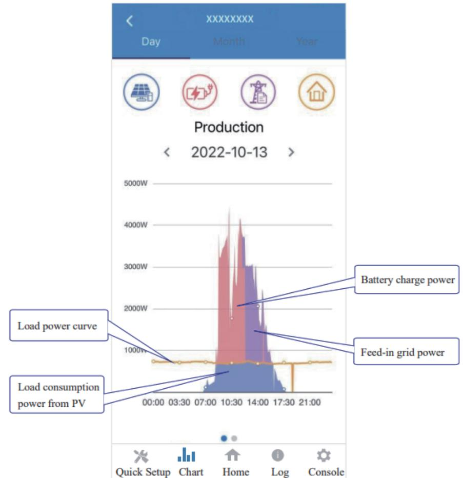
The above combination day chart shows the PV production power distributed with three parts: load consumption power (Blue) battery charge power (Red) feed-in grid power (Purple)
